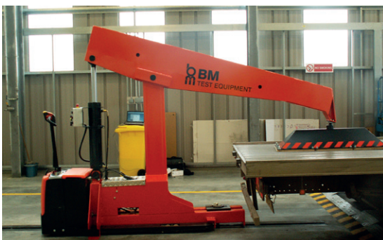
BM74000 - on-floor chassis load simulation
