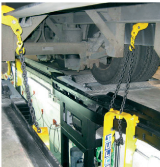
BM CLS Type A - pit wall mounting
